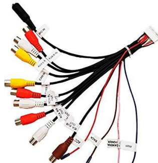
Kabelbund: (AUX-IN, CAM-IN, Mikrofön-IN, SUB-OUT, 4 x Audio-Out, ACC, Kamera Power, Back, AMP)
